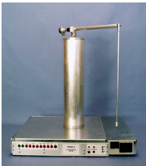
Figure 6.12 The Furuta pendulum.
